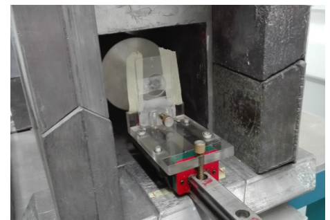
Figure 3: The HPGe detector used for the analysis of the irradiated VERDI detectors.
