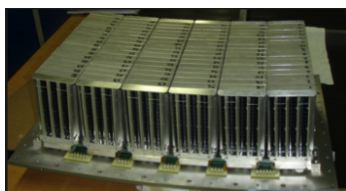
Fig. 4: A section of the Multi-Grid detector (32 cm x 48 cm). It can be scaled up to the areas required by chopper spectrometry.
